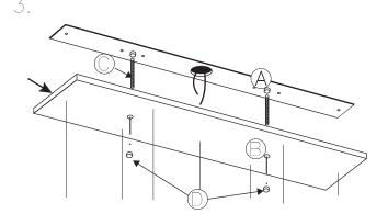
Complete attachment with button head screws  $\bigcirc$
